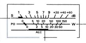
The second, "PO" scale indicates transmitter power output, in watts, when selected by the METER button in the depressed ( $\longrightarrow$  PO) position. This scale is calibrated to be most accurate when the antenna impedance is 50- $\Omega$ . Refer only to the numbers above the scale (0 - 150) for the FT-840: the numbers below apply only to special low-power versions.
