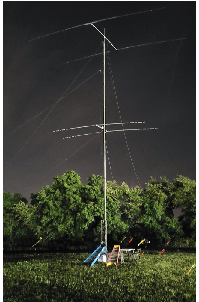
The Gloucester County Amateur Radio Club, W2MMD, in New Jersey, operated at night during the 2021 ARRL Field Day, with antennas for the 15-, 20-, and 80-meter CW stations. The antennas were supported by a portable aluminum military mast, which takes about an hour to deploy. [Vincenzo Sallustio, N4NYY, photo]
