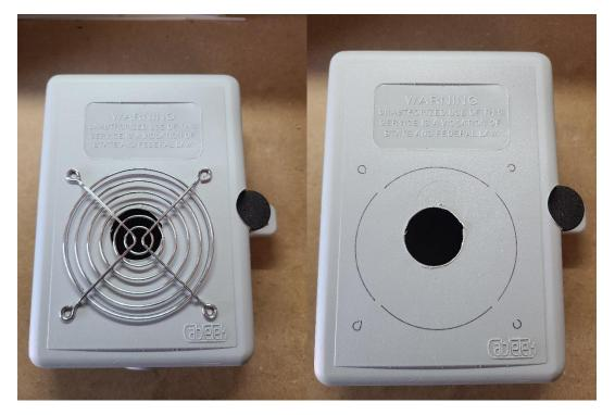
Mount the fan and grill to the CableTec enclosure front. Install Spade connectors to the fan power cord.
