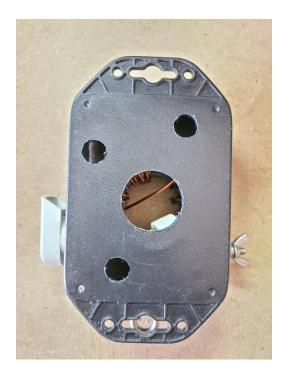
Mark the back of the CableTec enclosure to mount the MyAntennas Case on standoff spaceers
