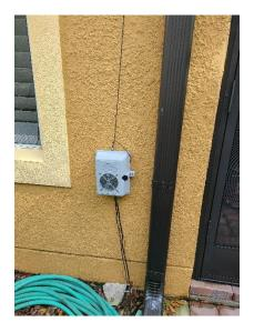
With this setup I have been able to transmit for extended time at 600 Watts on CW with absolutely no change in SWR. I believe this is a relatively inexpensive way to get the true power rating out of your end fed matching transformers.
