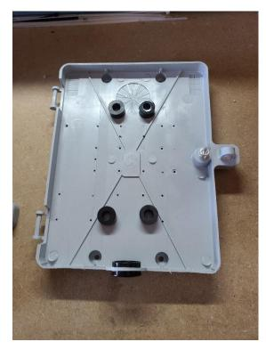
Drill some holes thru the back of the CableTec enclosure. Try to align the holes with those drilled in the rear of the MyAntennas case. Cover the holes with the heat-setting screen. Note I hand't finished the screening step in the photo below.
